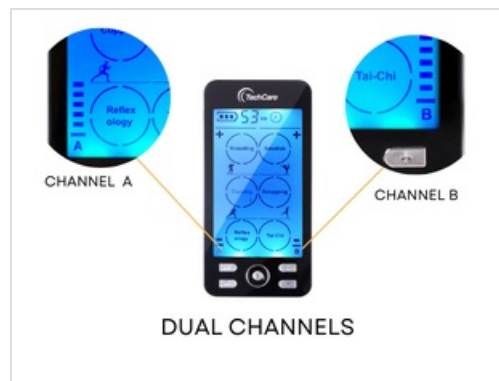
Image 6.4: The device's dual channel capability, allowing independent control for two sets of electrodes.
