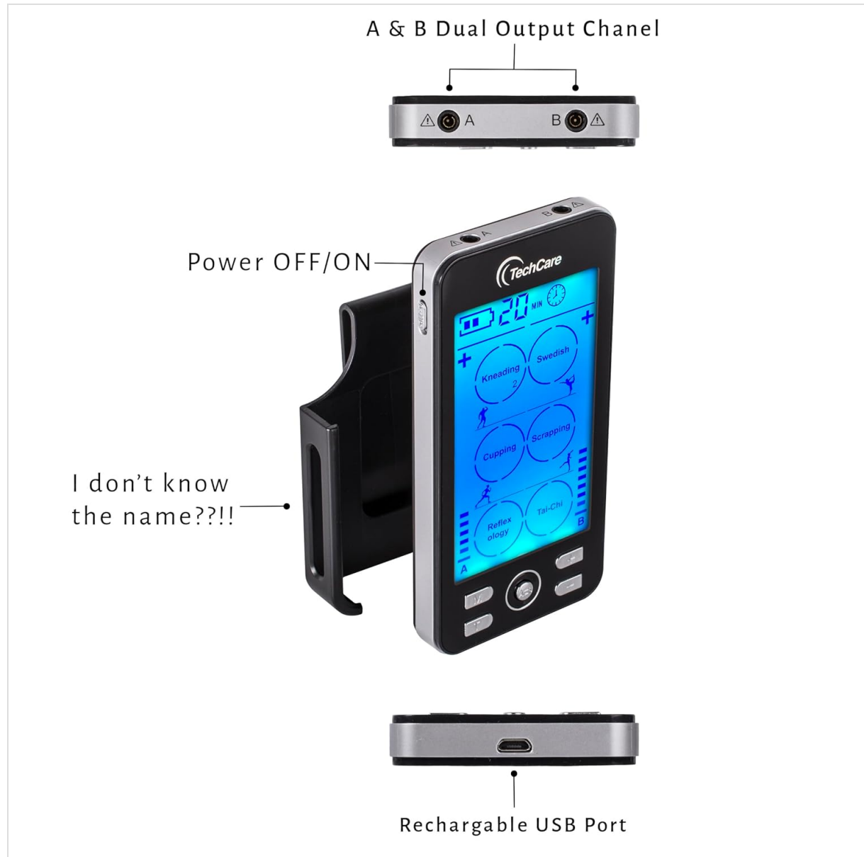
Image 4.1: Top, side, and bottom views of the device highlighting the dual output channels (A & B), the power switch, and the USB charging port.
