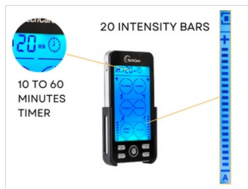
Image 6.3: The device's timer function, allowing sessions from 10 to 60 minutes.
