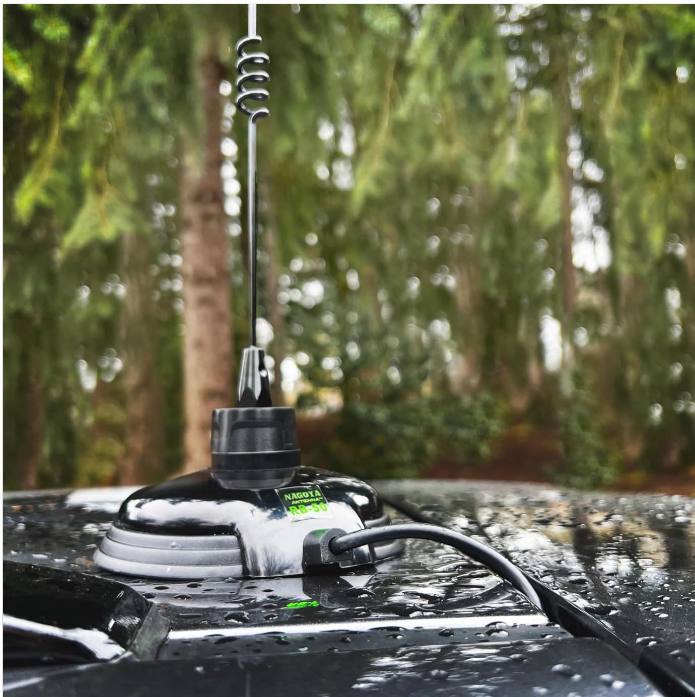
Figure 3: The RB-50 magnet mount with an NMO antenna installed on a vehicle roof.
