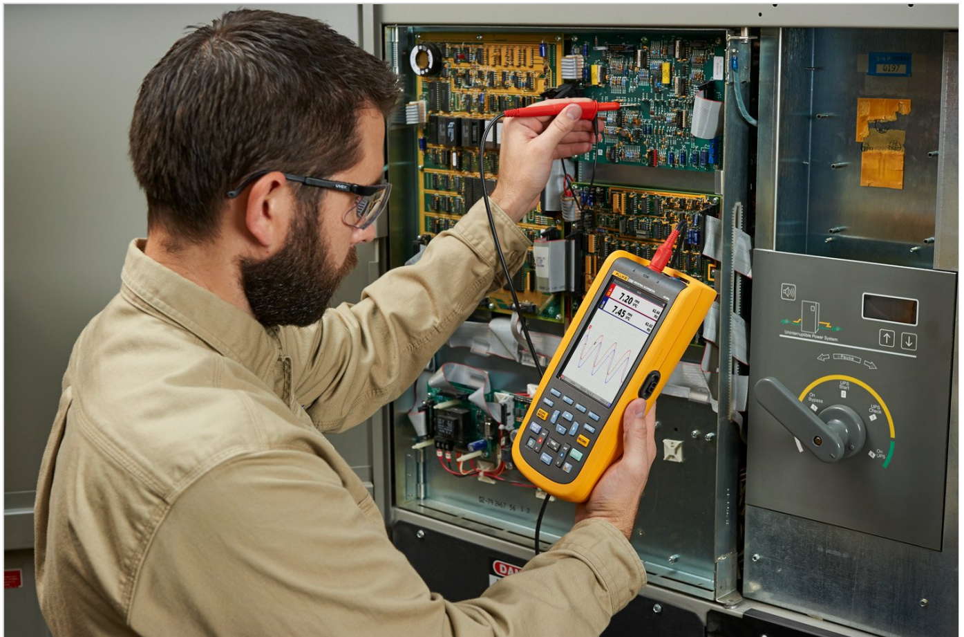
Figure 5.1: A technician actively using the Fluke 123B ScopeMeter to perform measurements within an electrical control panel, demonstrating its application in industrial environments.
