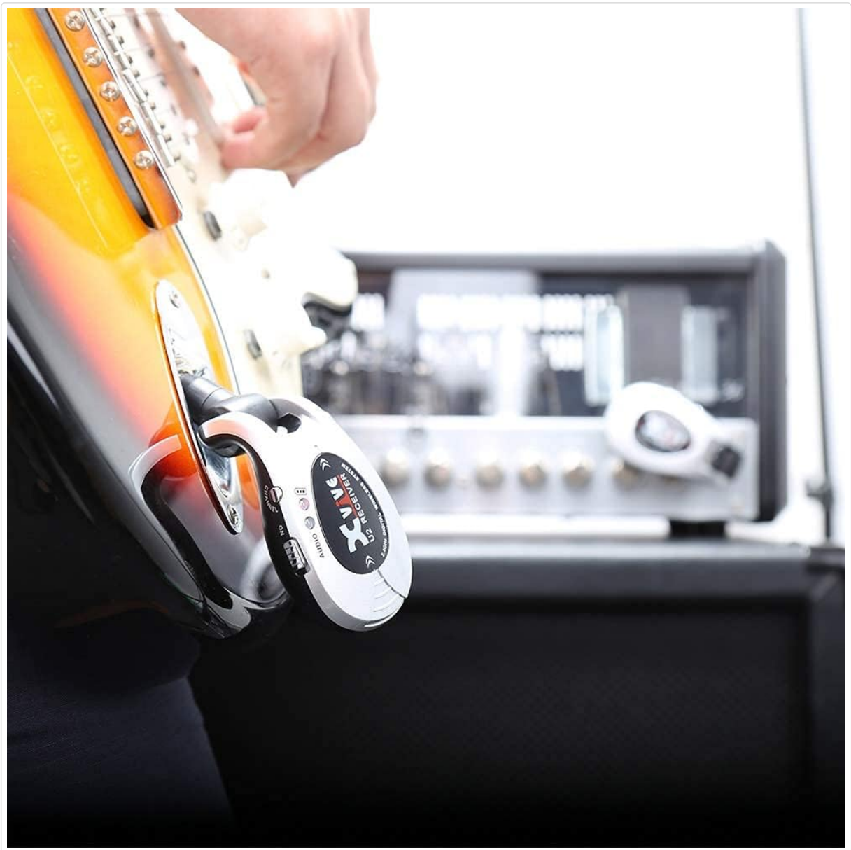
Figure 3: The Xvive U2 Transmitter connected to an electric guitar.
