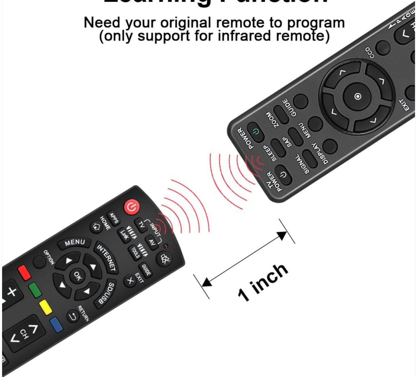
Figure 3.2: The remote's learning function allows it to mimic commands from your original infrared remote.
