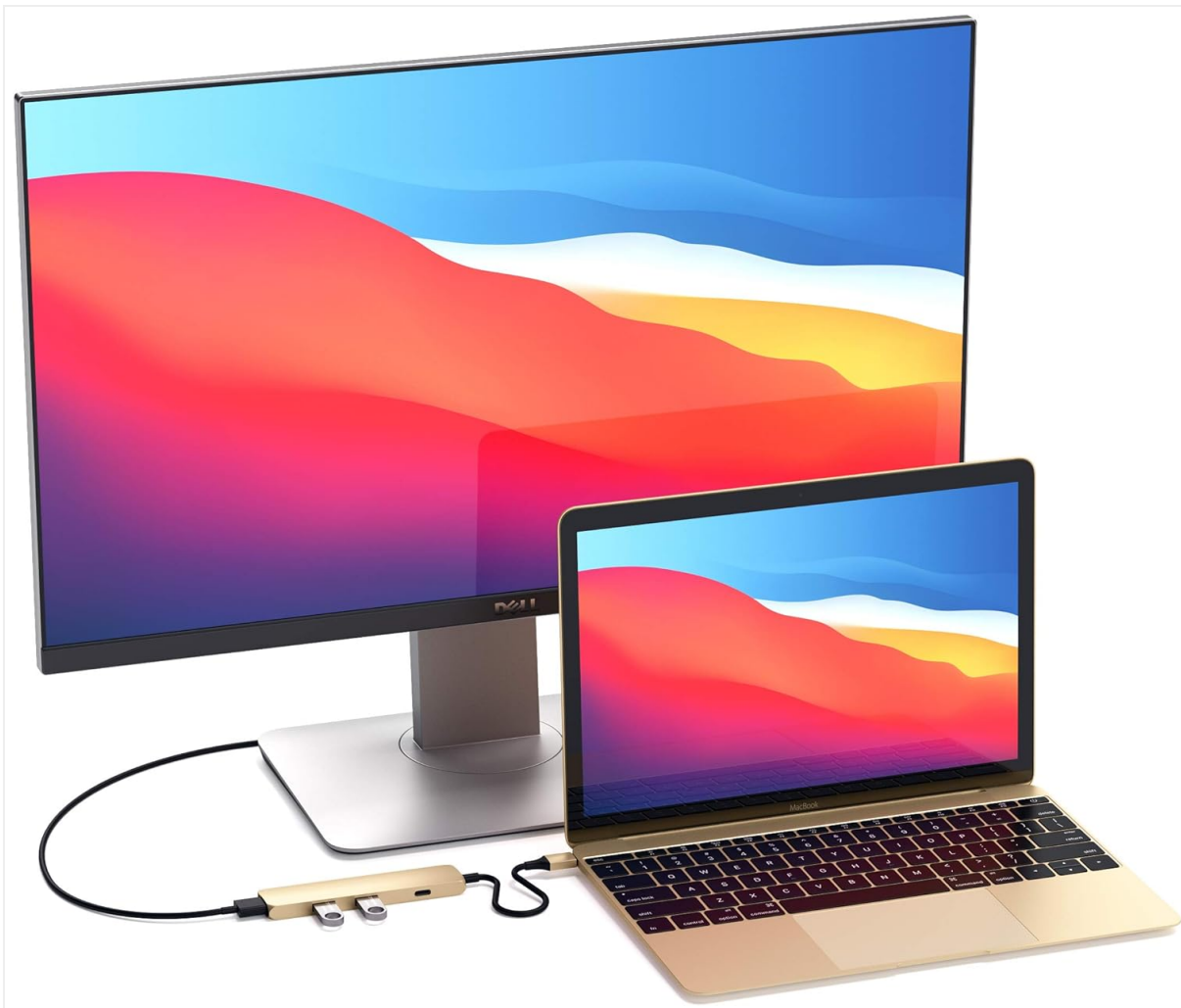
Image 3.1: Hub connected to a MacBook and external display. This image illustrates the hub facilitating an extended display setup, with the MacBook connected to a larger monitor via the hub's HDMI port.
