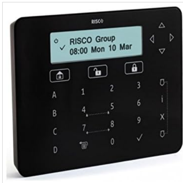
Figure 1: Risco Rokkonet Touch Elegant Keypad. This image displays the Risco Rokkonet Touch Elegant Keypad in black. The central display shows 'RISCO Group' and '08:00 Mon 10 Mar'. Below the display are touch-sensitive buttons including numeric keys (0-9), alphabetical keys (A-D), and function icons for home, unlock, lock, navigation arrows, checkmark, and 'X'.
