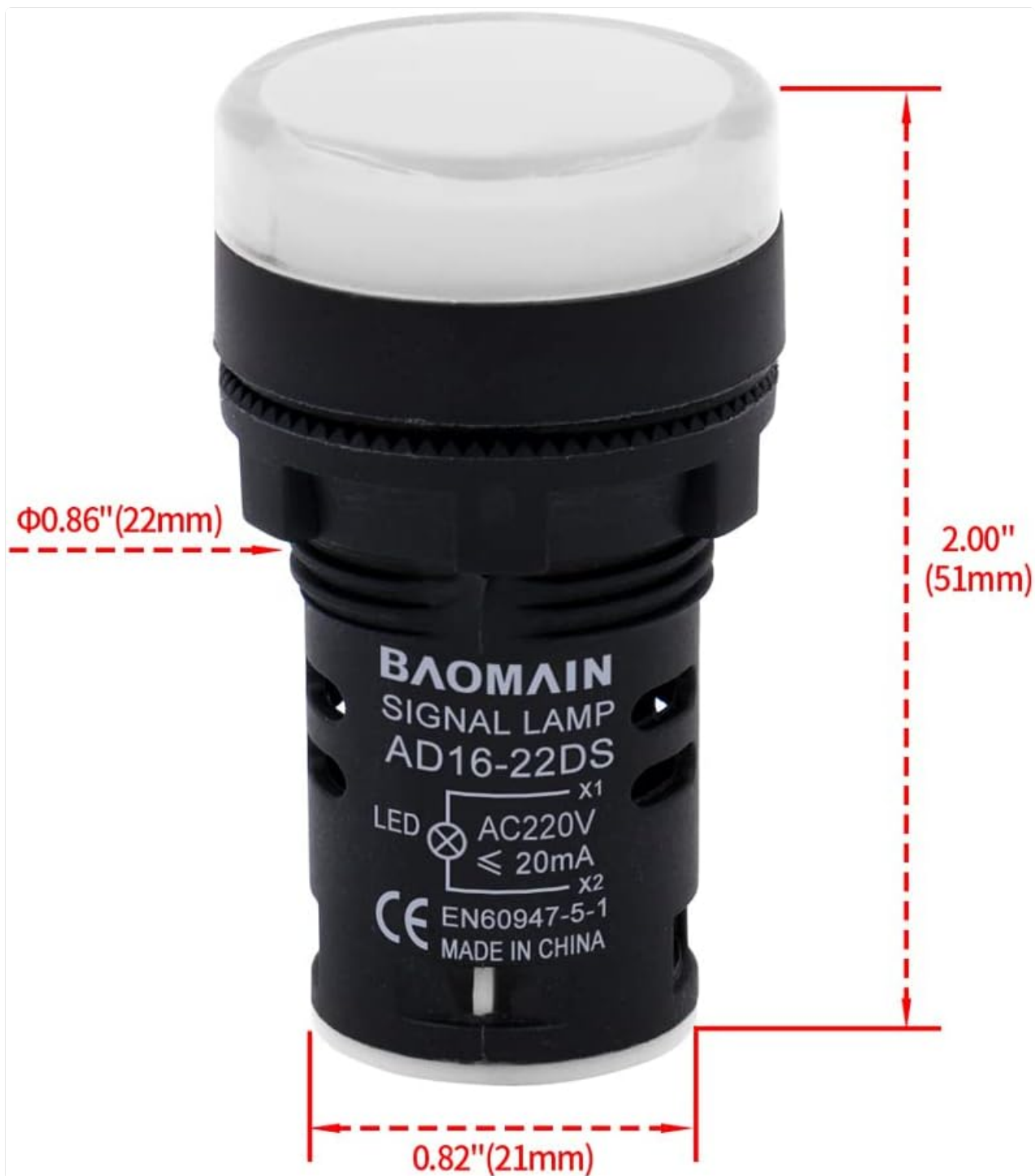
Figure 8.1: Dimensional drawing illustrating the key measurements of the Baomain AD16-22D indicator light, including the 22mm mounting diameter, 50mm (2.00") length, and 21mm (0.82") base diameter.
