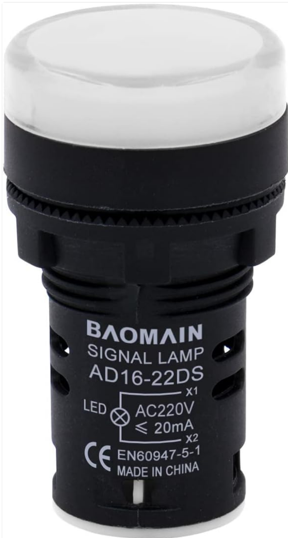
Figure 3.1: A detailed view of the Baomain AD16-22D indicator light, showing the branding, model number, LED type, voltage rating (AC220V), current rating ( \leq 20\text{mA} ), and compliance markings (CE, EN60947-5-1).
