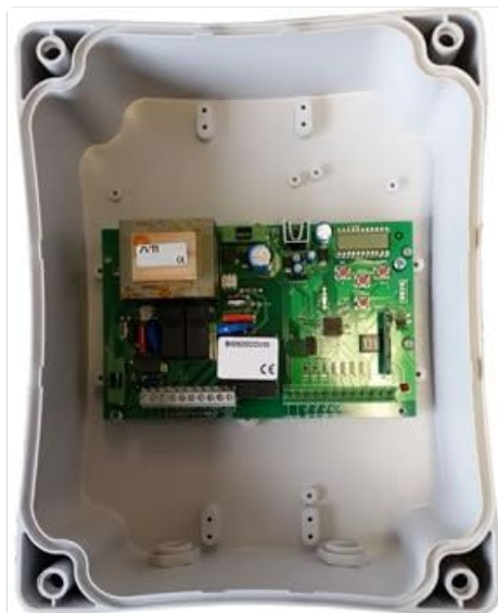
Figure 2: Detailed internal view of the control unit, providing a closer look at the electronic components and connection points for various gate accessories.
