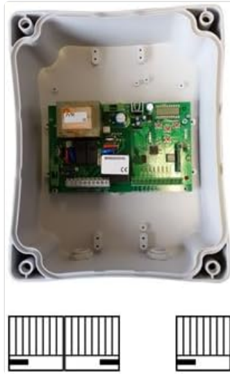
Figure 1: Internal view of the ALLMATIC BIOS2 Eco control unit, showing the main circuit board, transformer, and terminal blocks within its protective enclosure.
