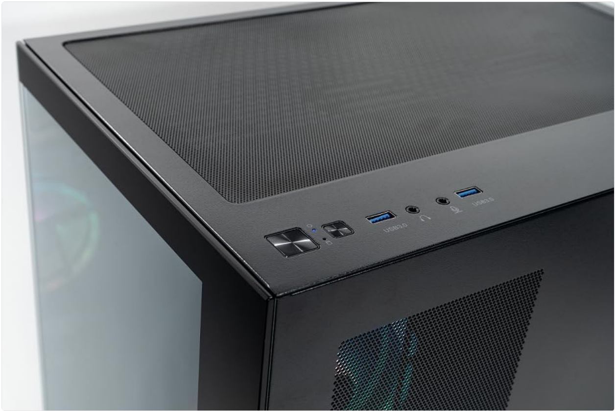
Image 2.2.2: Top panel of the CYBERPOWERPC Luxe Gaming PC. This image highlights the power button, reset button, two USB 3.0 ports, and audio input/output jacks located on the top of the PC case for easy access.
