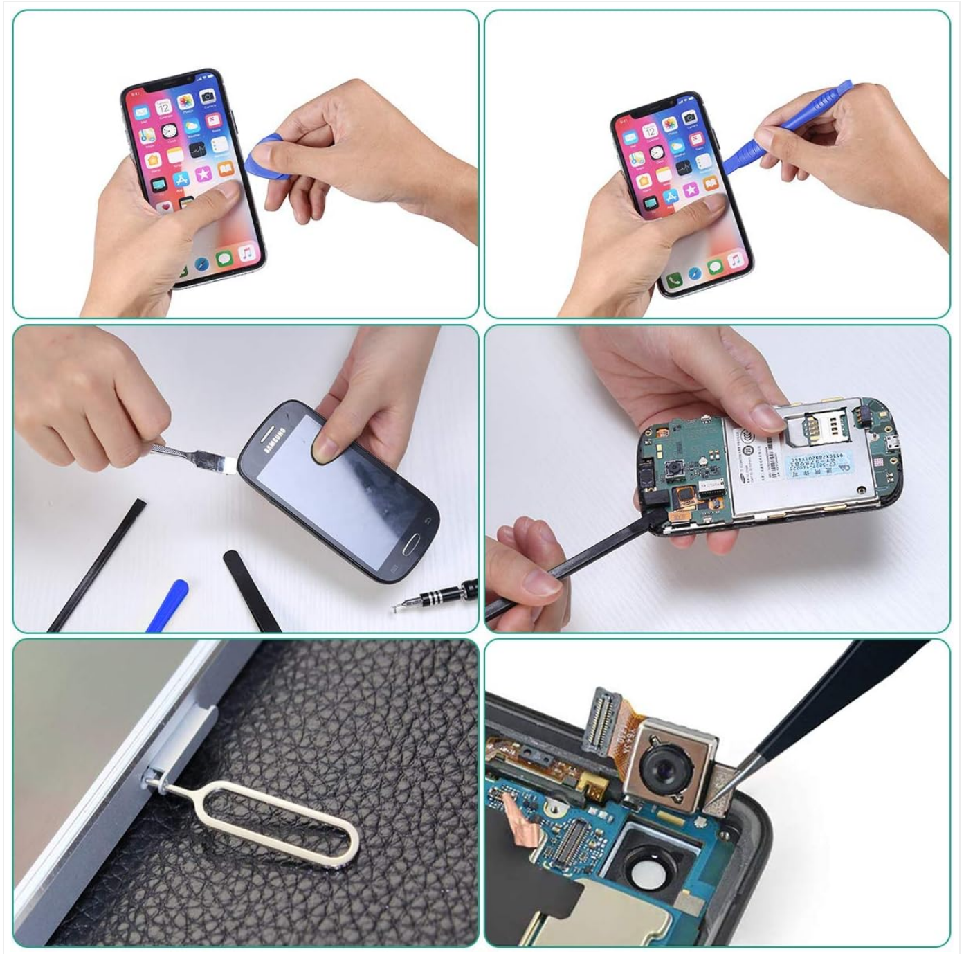
Figure 4.1: Illustrates various repair scenarios including prying open a phone, handling internal components, and using the SIM ejector tool.
