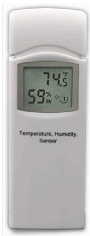
Figure 2: A single remote thermo-hygrometer sensor. These sensors transmit temperature and humidity data wirelessly to the main console.
