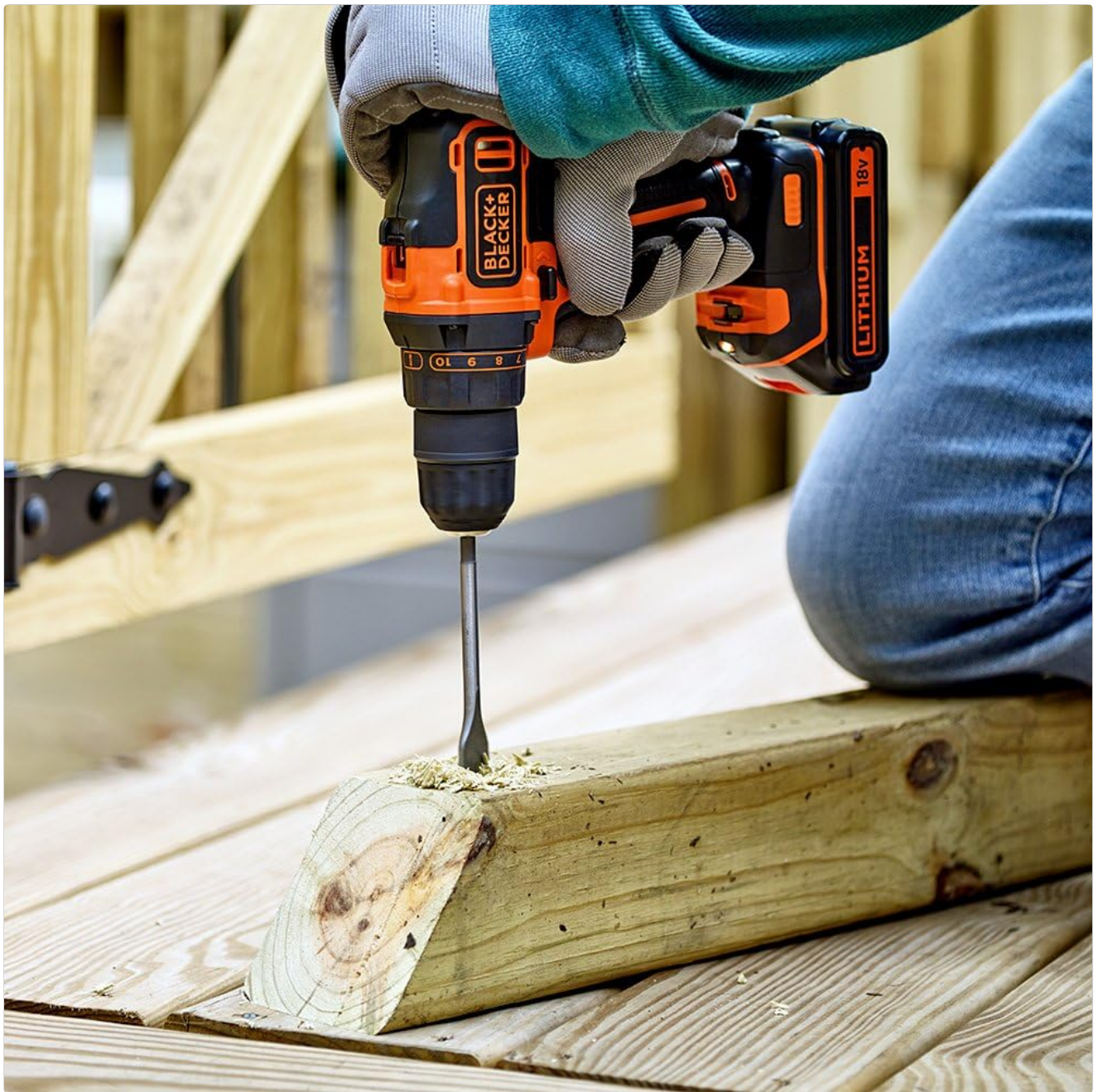
Image: A person using the BLACK+DECKER 18V Cordless Drill Driver to drill a pilot hole into a wooden beam on an outdoor deck. The drill is held firmly, and wood shavings are visible around the drill bit.
