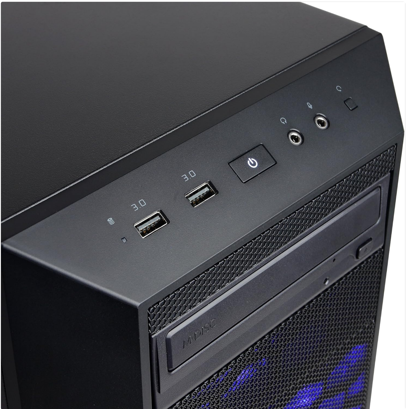
Figure 2.2: Front I/O panel showing USB 3.0 ports, headphone/microphone jacks, and the power button.
