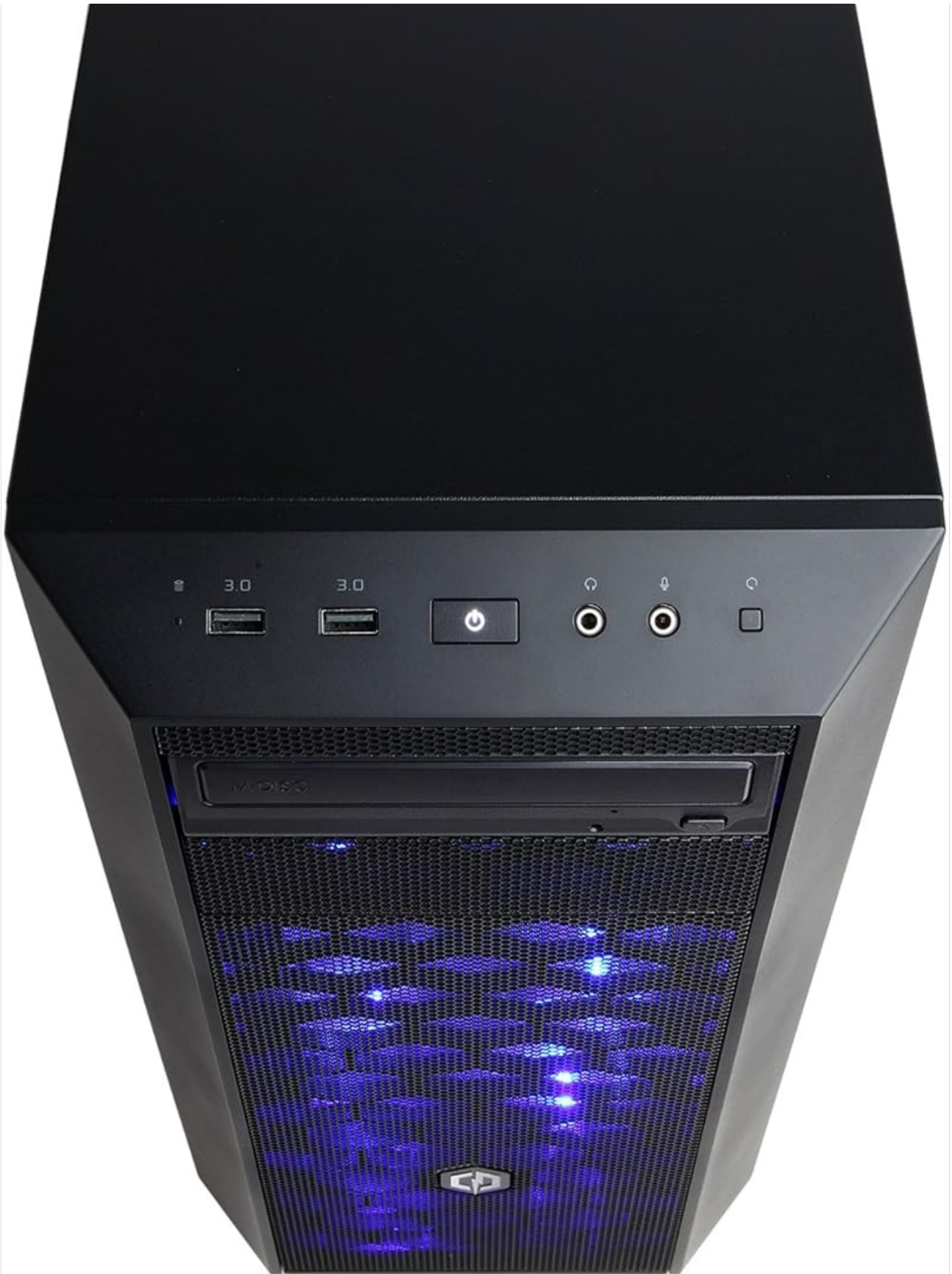
Figure 2.3: Top-down view of the PC, illustrating the layout of the front panel ports and the top exhaust fan.
