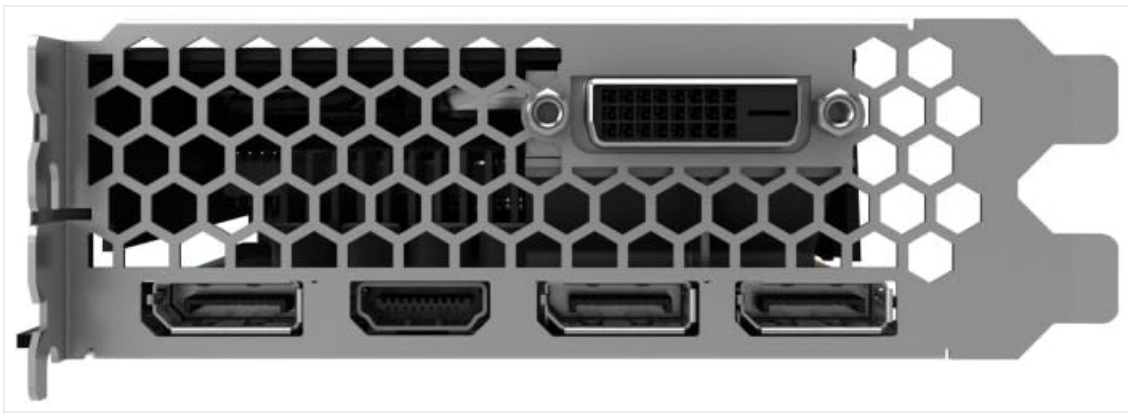
Figure 5.2: Rear view of the graphics card with DVI, HDMI, and DisplayPort outputs.
