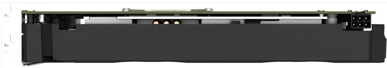
Figure 5.1: Side view of the graphics card, highlighting the 6-pin power connector.
