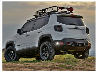
Figure 4.4: Rear view of a white Jeep Renegade with the RIGID Ignite LED Diffused Flush Mount Light illuminated. The light is visible on the rear bumper, casting a bright, wide beam, illustrating its effectiveness as an auxiliary reverse or area light.
