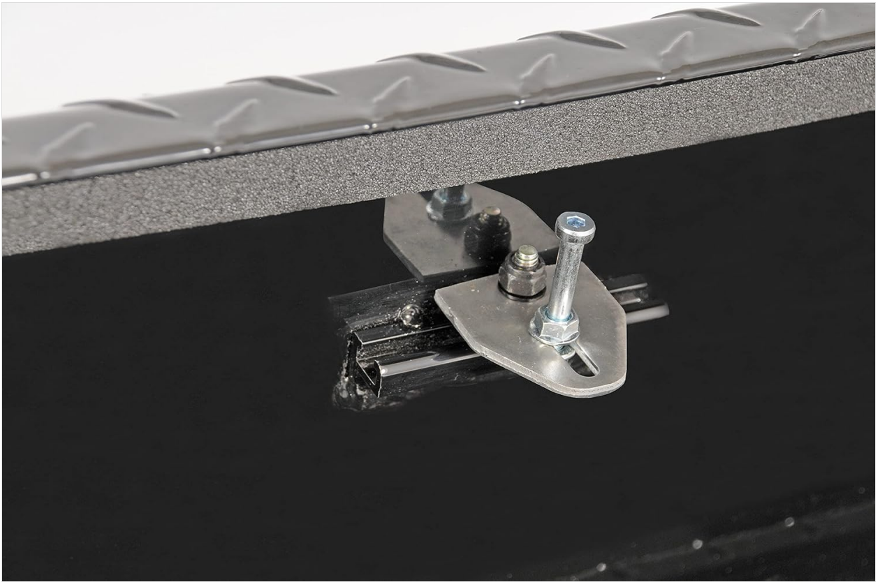
Image: Close-up view of the mounting hardware, showing bolts and brackets used to secure the tank to the truck bed.
