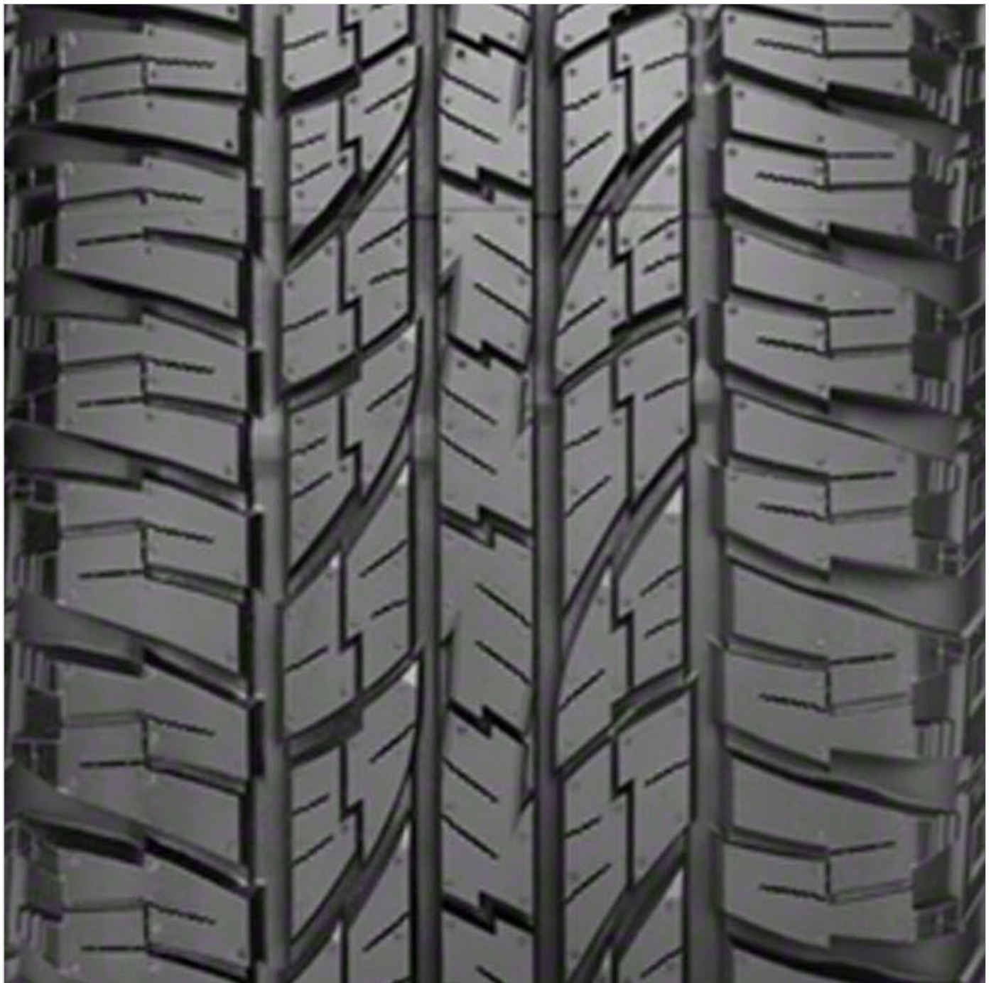
Figure 5.1: Close-up view of the Yokohama Geolandar AT G015 tire tread, highlighting the siping and block design for traction.
