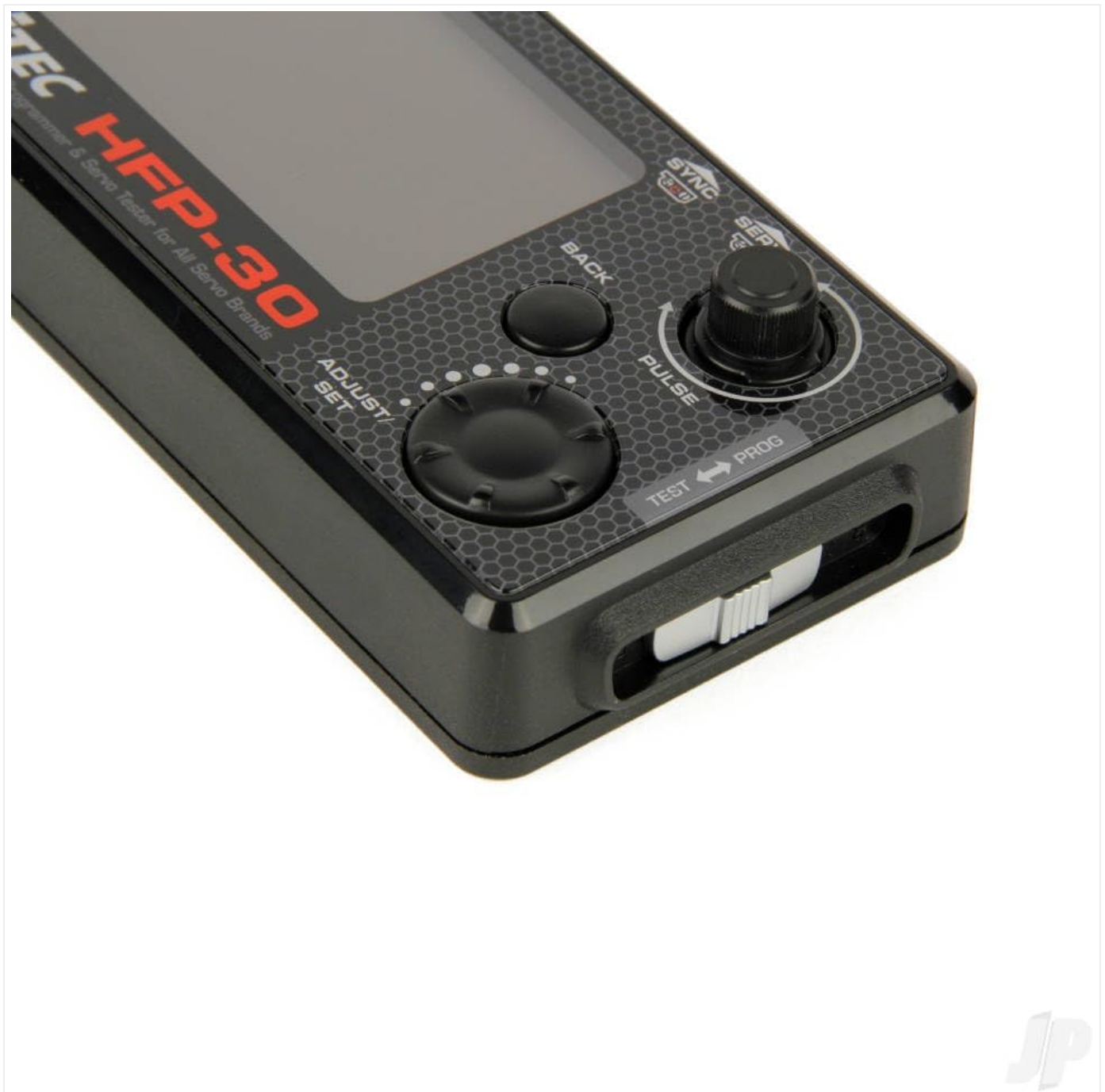
Figure 3.2: Close-up view of the control panel on the Hitec HFP-30. Visible controls include a rotary knob labeled "ADJUST/SET", a button labeled "BACK", another rotary knob labeled "PULSE", and a switch to toggle between "TEST" and "PROG" modes. Two servo ports are also visible.
