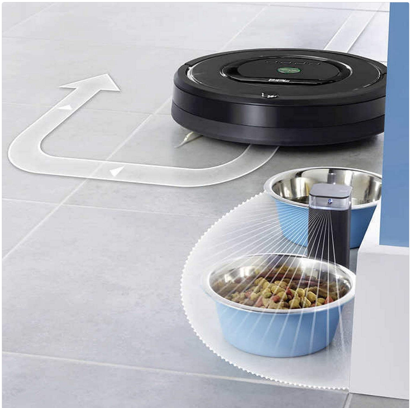
Image: The Roomba 805 utilizing its edge-sweeping brush to clean along the perimeter of a room or doorway.
