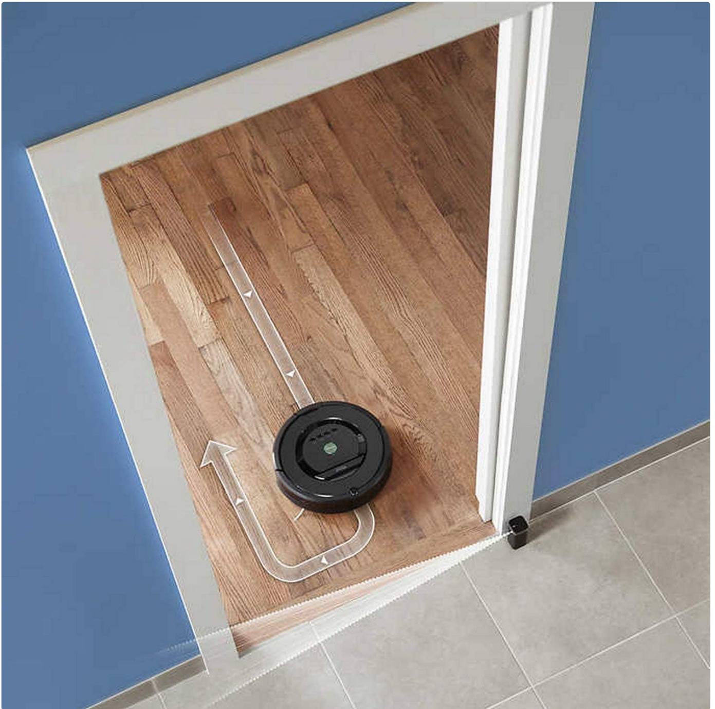
Image: The Roomba 805 detecting a drop-off, such as stairs, and adjusting its path to avoid falling.
