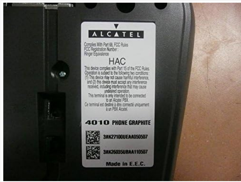
Figure 2: Close-up of the rear label on the Alcatel-Lucent 4010 phone. This label provides important regulatory information, including FCC compliance details, and identifies the model as "4010 PHONE GRAPHITE" along with QR codes for product identification.
