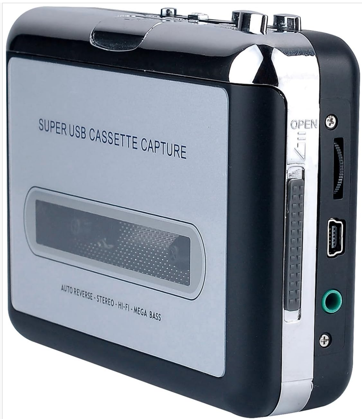
Figure 2: Side view of the ezcap218, highlighting the USB port, 3.5mm audio output, and volume control.
