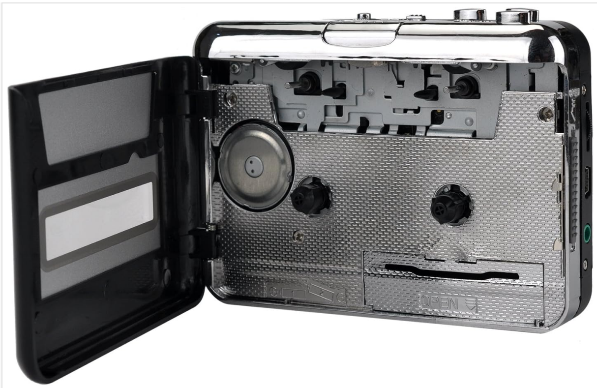
Figure 4: Inside view of the ezcap218 with the cassette compartment open, showing the tape mechanism.
