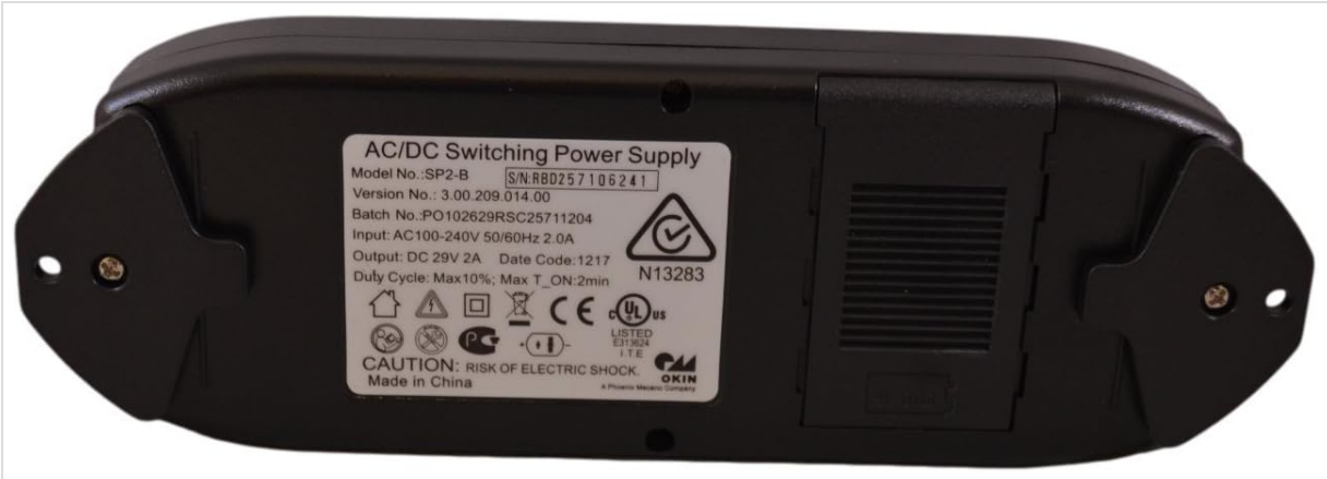
Figure 2: Rear view of the power supply unit, displaying the model number, input/output specifications, and safety certifications.
