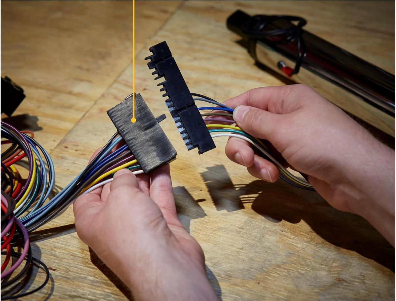
Figure 5: Demonstration of connecting the GM column wiring plug, illustrating the plug-and-play design for compatible steering columns.
