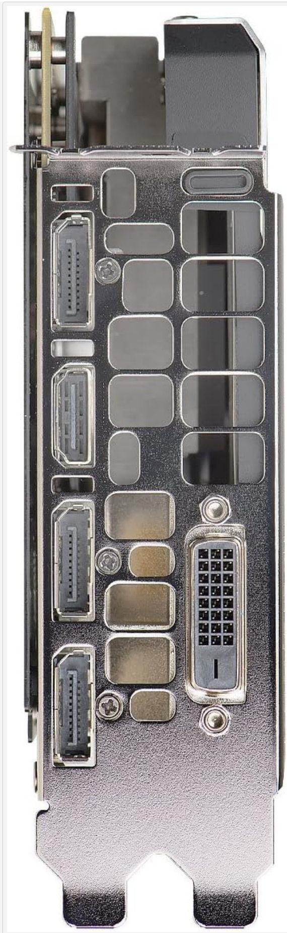
Image: Rear I/O panel of the graphics card, showing DisplayPort, HDMI, and DVI outputs.
