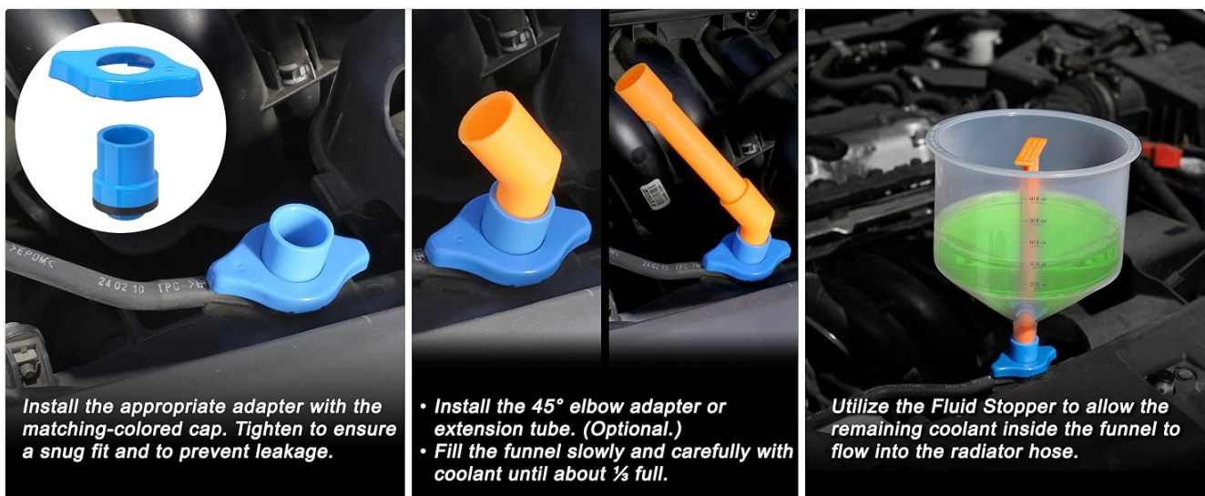
Figure 3.1: Visual instructions for installing the correct adapter, optional extensions, and the funnel onto a radiator.
