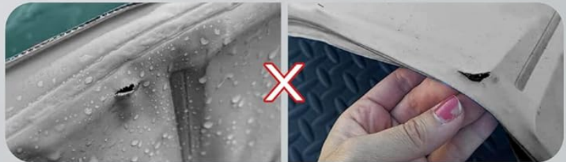
Holes and tears along the edges
