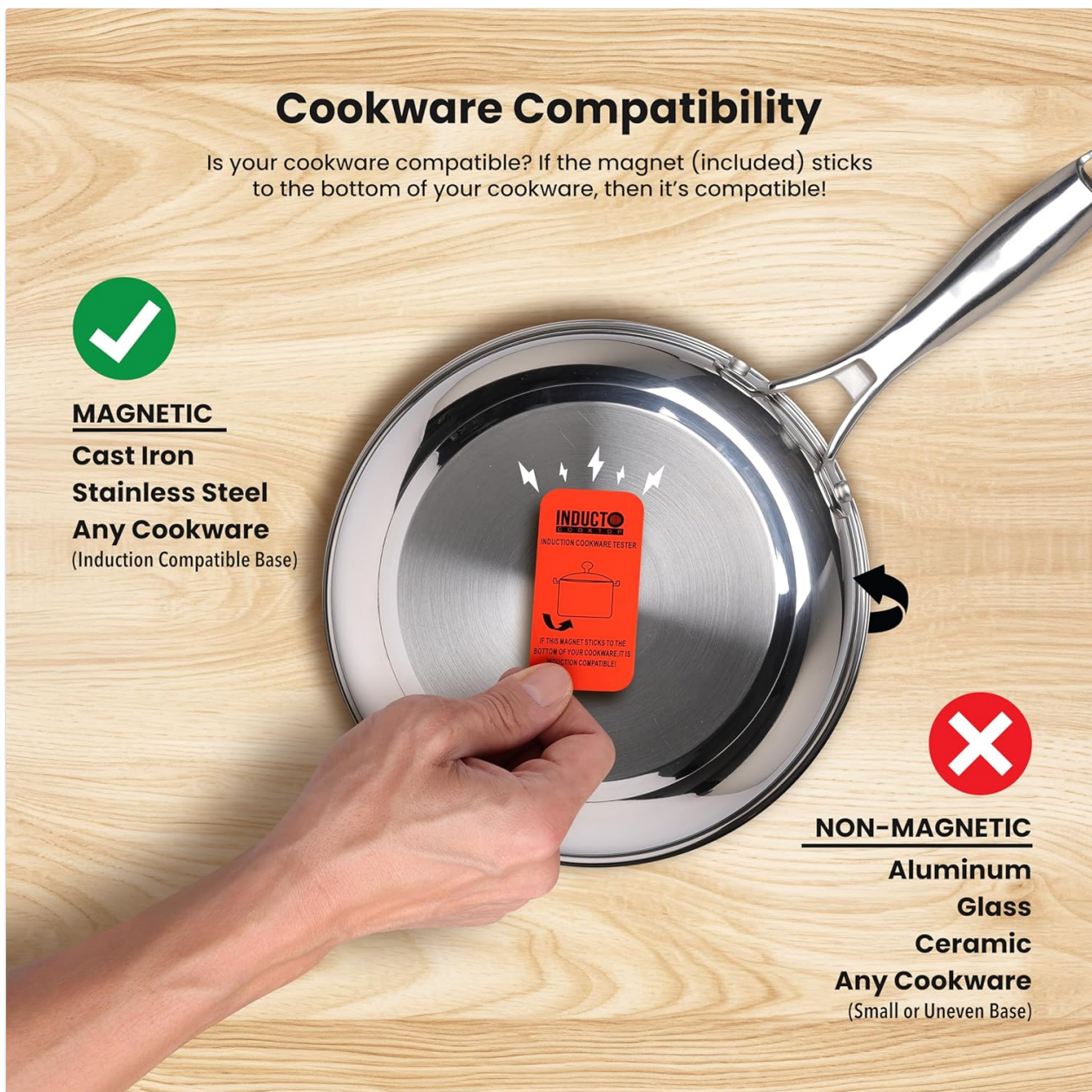
Figure 3.1: Cookware Compatibility Test. This image illustrates how to use a magnet to determine if a pot or pan is suitable for induction cooking. If a magnet sticks firmly to the bottom, the cookware is compatible.
