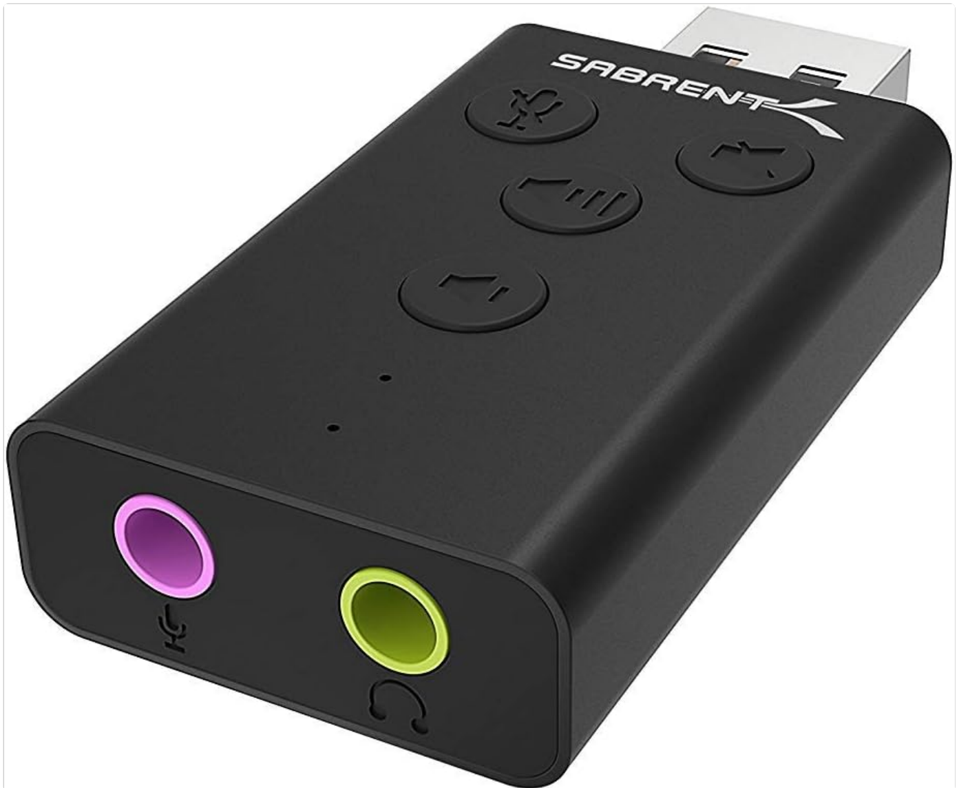
Image: Close-up view of the SABRENT AU-DDAB adapter, highlighting the green audio output jack and pink microphone input jack.
