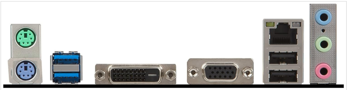
Figure 2.2: Detailed view of the motherboard's rear input/output (I/O) ports, including USB, audio, and video outputs.
