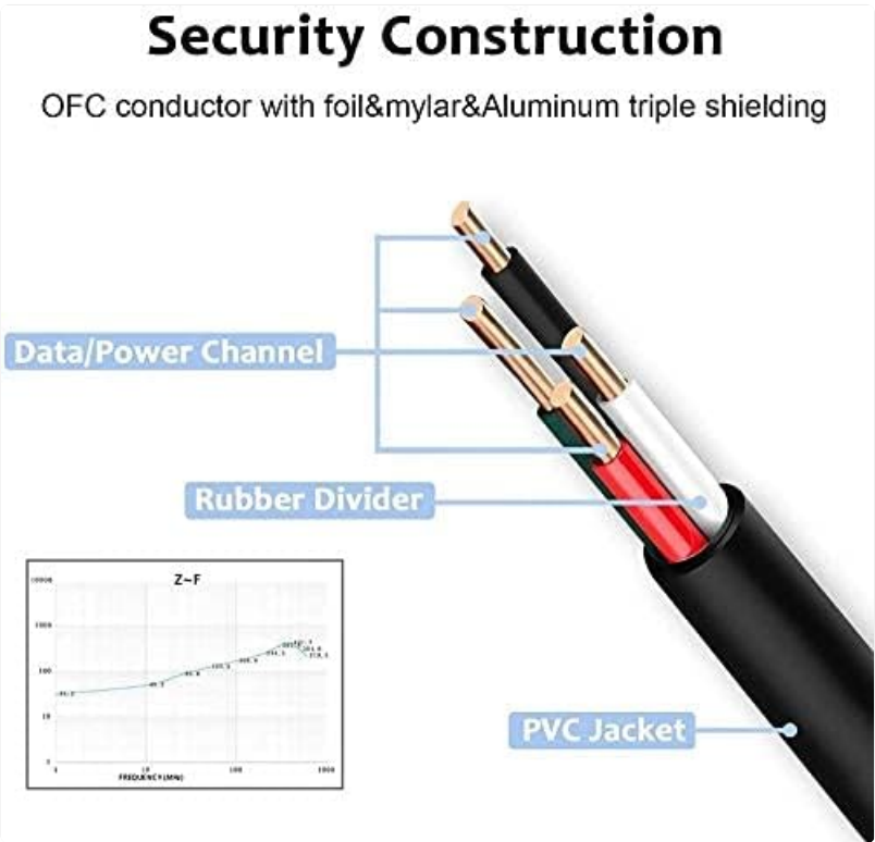
Image: Cable Internal Construction
