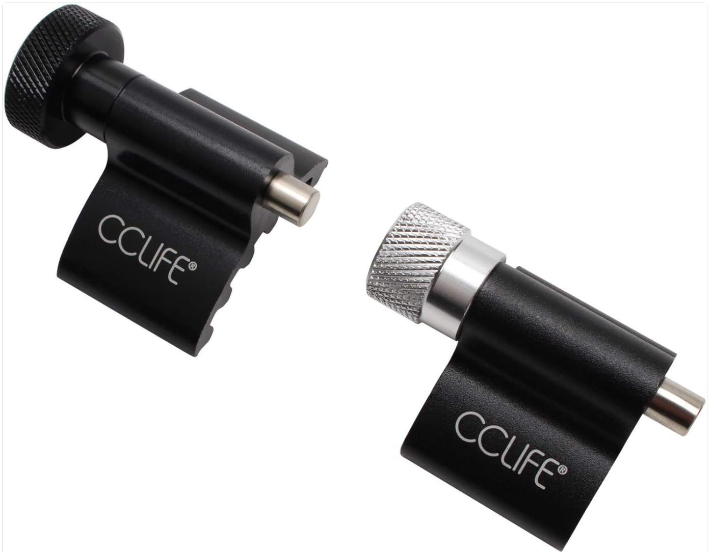
Image 3.3: Detailed view of the two crankshaft locking tools (T10050 and T10100).
