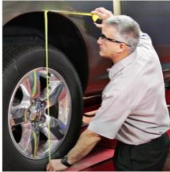
Image 5.6: Measuring ride height after installation to confirm proper restoration.
