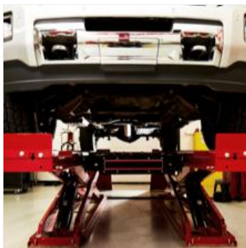
Image 5.2: Vehicle properly secured on a lift for suspension service.
