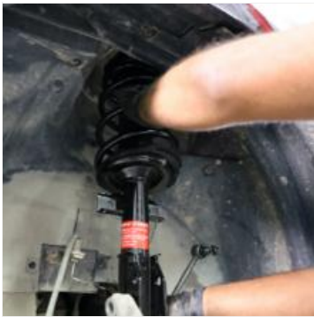
Image 5.3: A new strut assembly being carefully positioned for installation.
