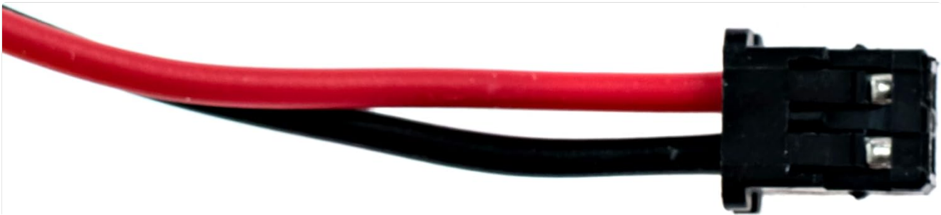
Image 5.1: Close-up view of the battery connector, showing the red and black wires.
