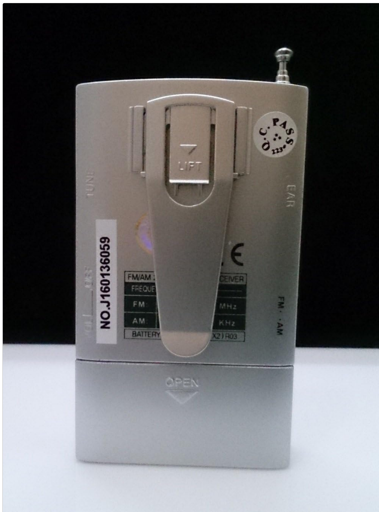
Image: Back view of the Sami RS 2912 radio, highlighting the battery compartment cover and the integrated belt clip.
