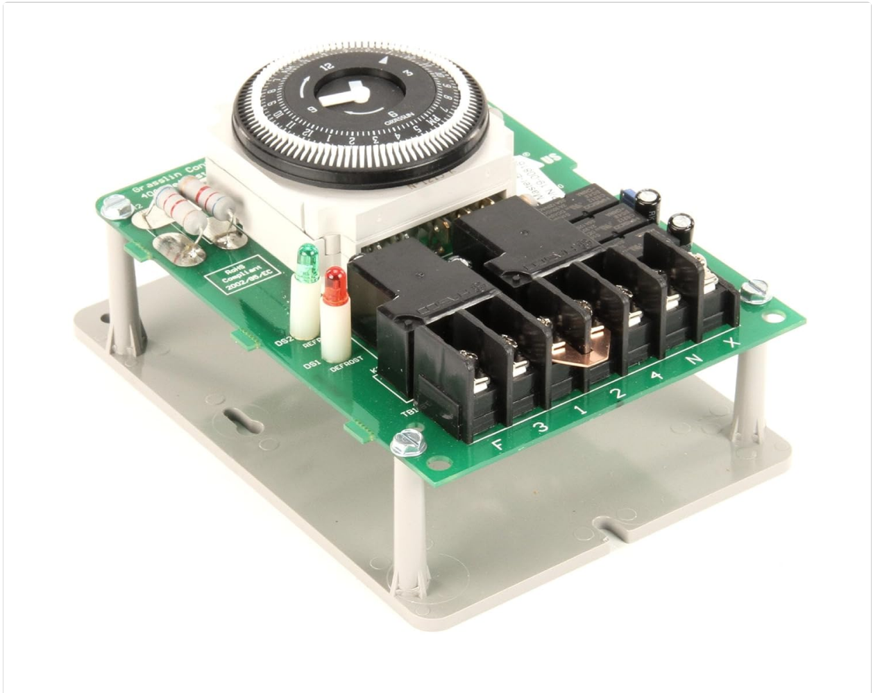
Figure 4.1: View of the timer unit highlighting the electrical terminal blocks. This image shows the screw terminals where system wiring connects to the timer unit for power and load control, with labels like F, 3, 1, 2, 4, N visible.
