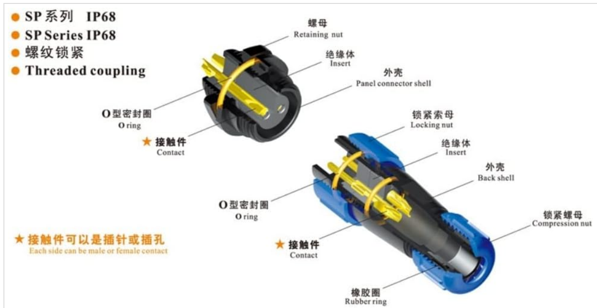
Figure 3.2: Exploded view illustrating the internal components of the SP21 connector, including the retaining nut, insert, panel connector shell, locking nut, back shell, compression nut, O-rings, rubber ring, and contacts.
