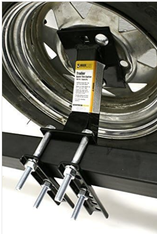
Figure 3: The spare tire carrier installed on a trailer tongue.
