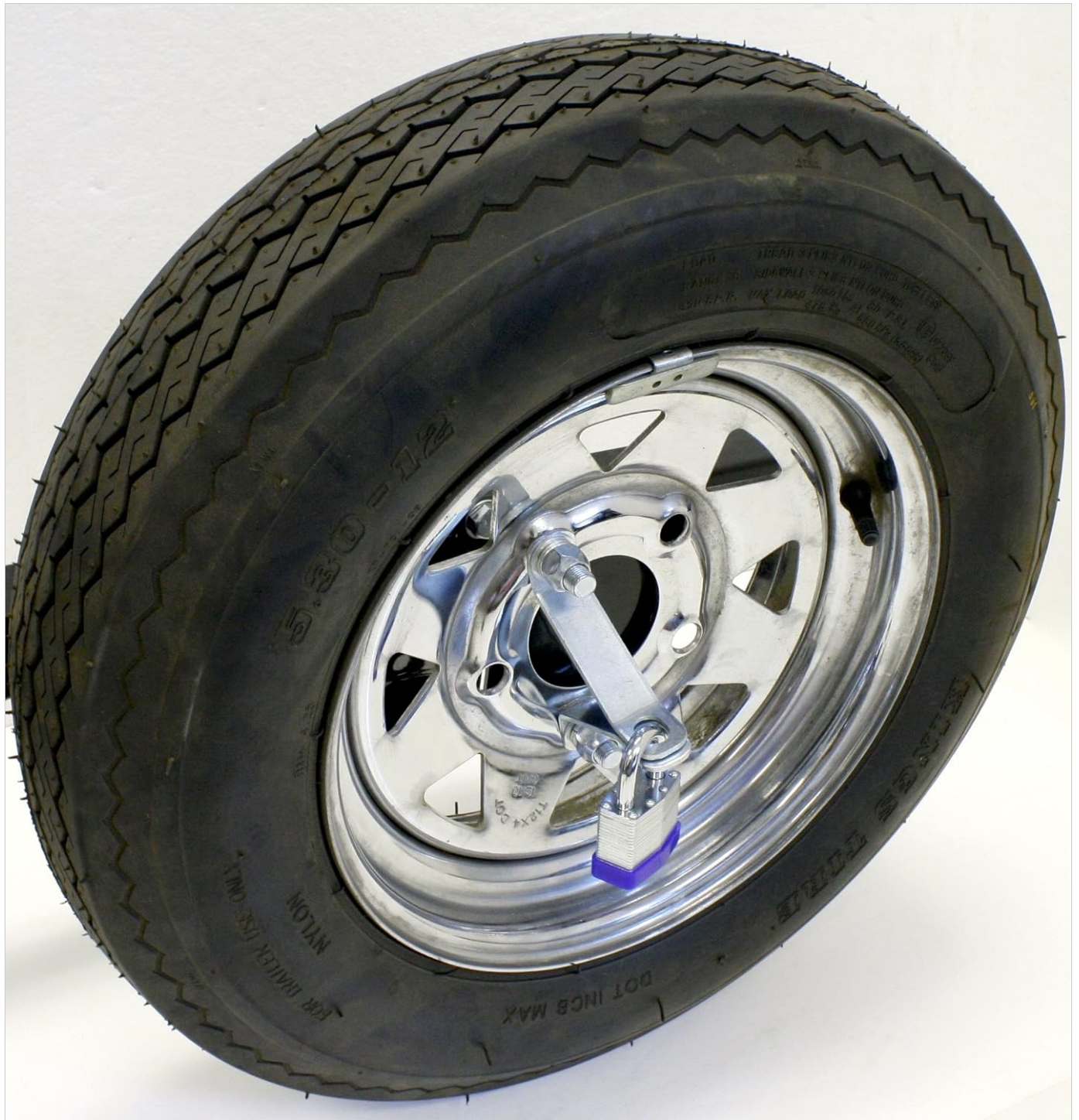
Figure 4: Spare tire mounted on the carrier, secured with the locking bracket.
