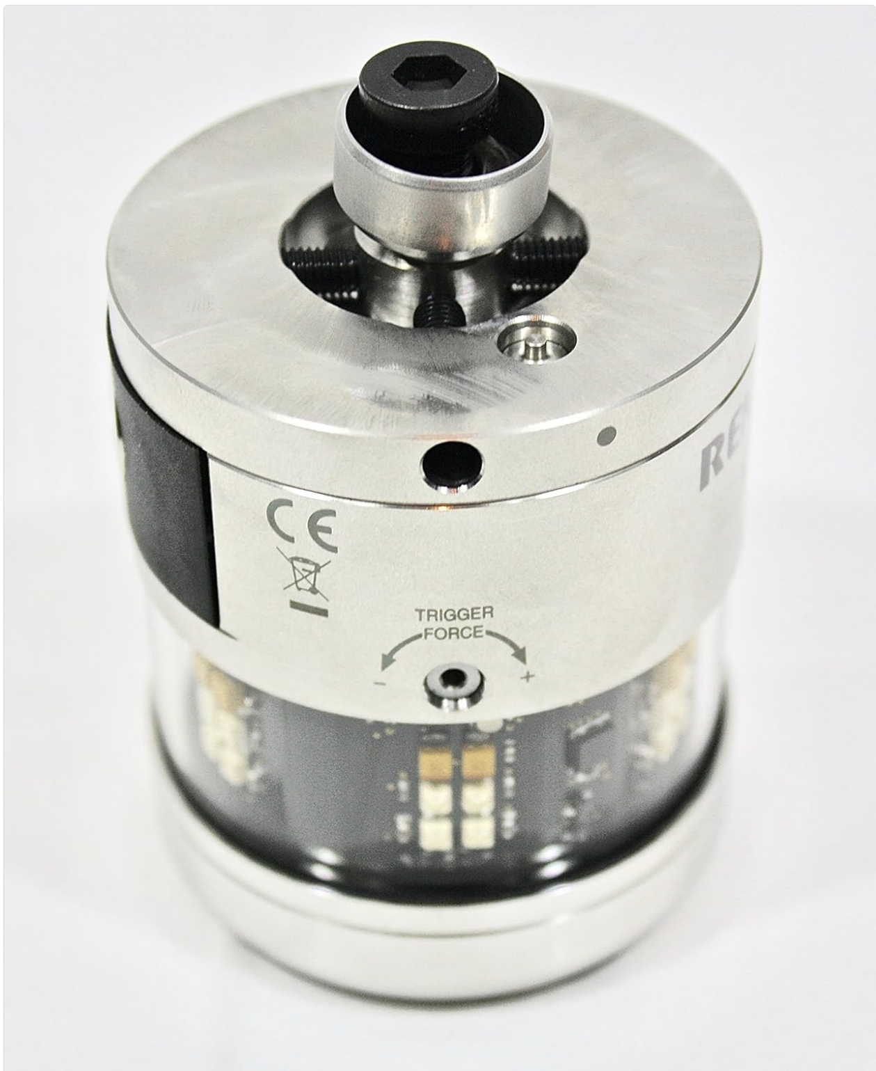
Image: A close-up view of the Renishaw OMP60 probe, indicating the 'TRIGGER FORCE' adjustment screw with directional arrows for increasing or decreasing the trigger force. This adjustment allows fine-tuning of the probe's sensitivity.
