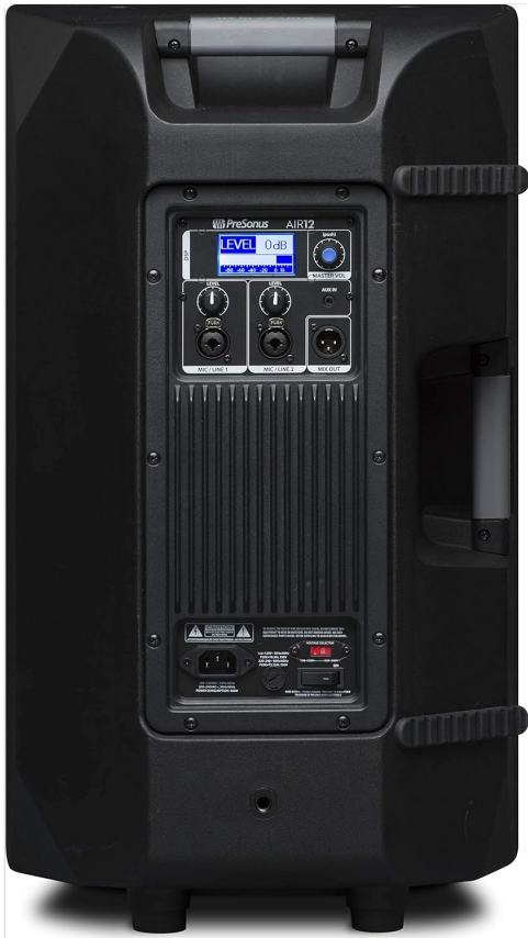
Figure 4: Rear panel of the PreSonus AIR12 loudspeaker, displaying input/output connections, level controls, and DSP preset selection. This panel is the central hub for all audio and configuration adjustments.
