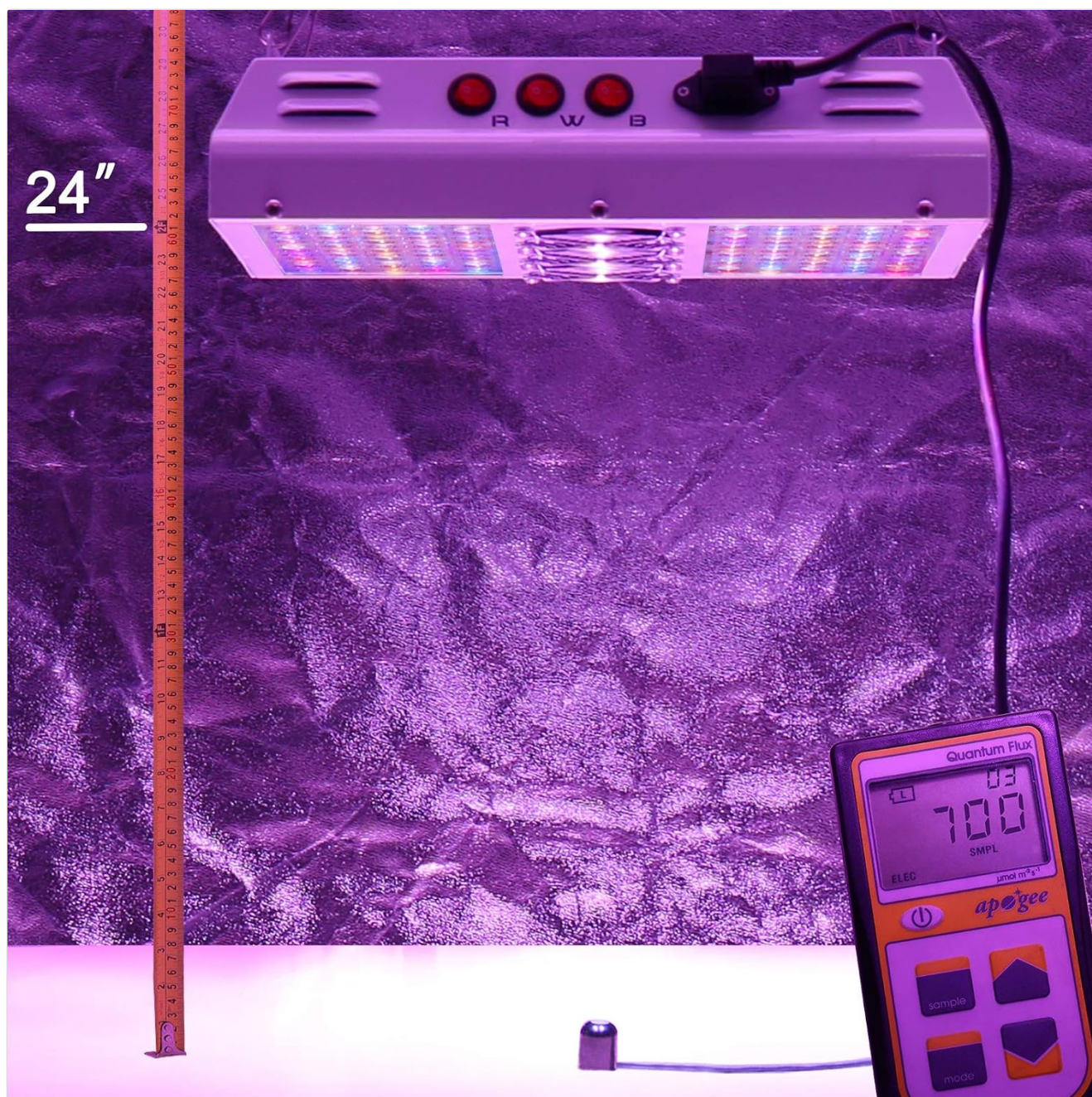
Figure 7.1: The PAR600 light positioned at a 24-inch height, demonstrating a PAR reading of 700 \mu\text{mol m}^{-2} \text{s}^{-1} at the center.
