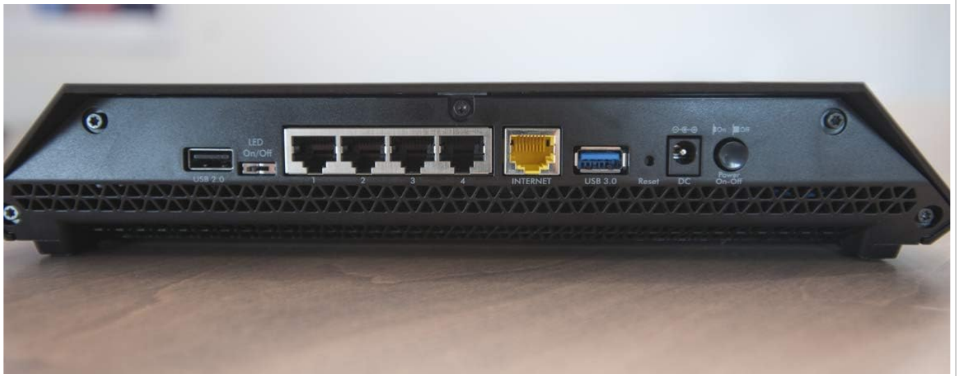
Figure 2: Rear panel of the Nighthawk X6S router with Ethernet, WAN, USB, and power ports.
