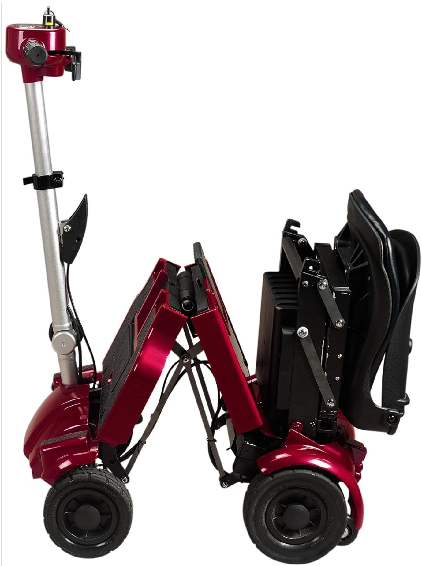
Image: The iLiving i3 Foldable Electric Scooter in a partially folded state, demonstrating its compact design for storage or transport.
