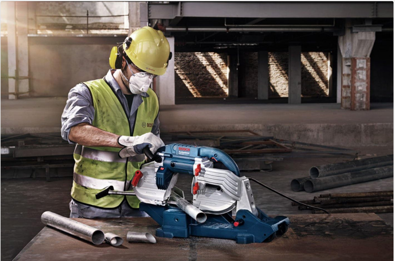
Figure 4.1: A user operating the Bosch GCB120B in its stationary configuration, demonstrating the stability provided by the base during cutting operations.
