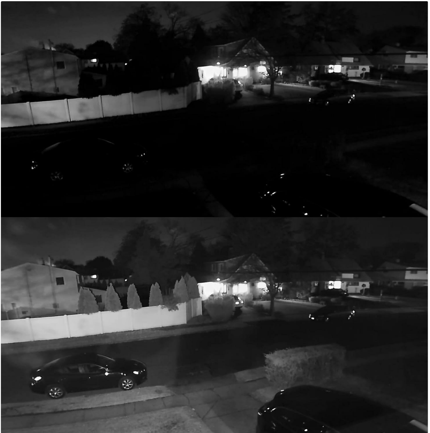
Image: A split image demonstrating the effectiveness of the IR illuminator. The top half shows a dark scene without IR light, while the bottom half shows the same scene clearly illuminated by the IR device, as seen through a night vision camera.
