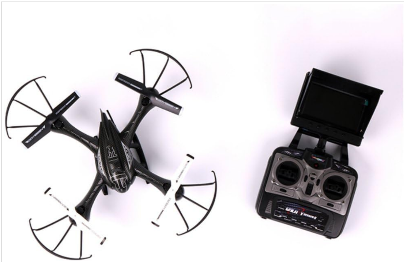
Image: The Galaxy Seeker II drone positioned next to its remote control. The remote control features dual joysticks and a top-mounted FPV screen for live video feed.
