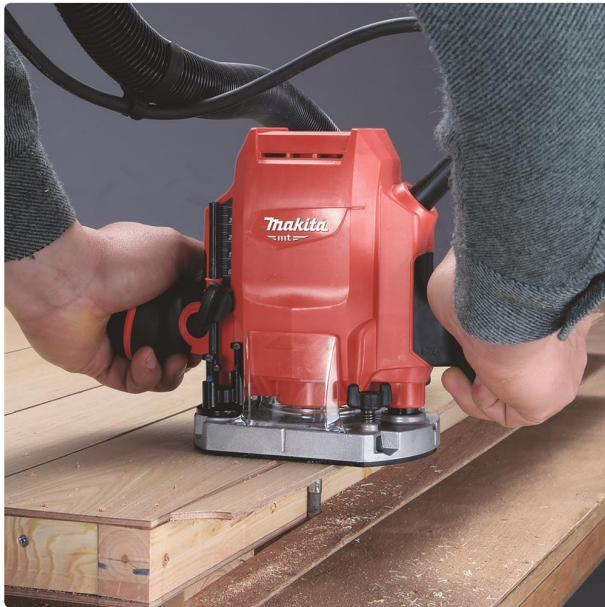
The Makita M3601 Electric Router being used on a wooden workpiece, demonstrating its application in routing operations. A dust collection hose is visible, indicating the tool's capability for dust management.
