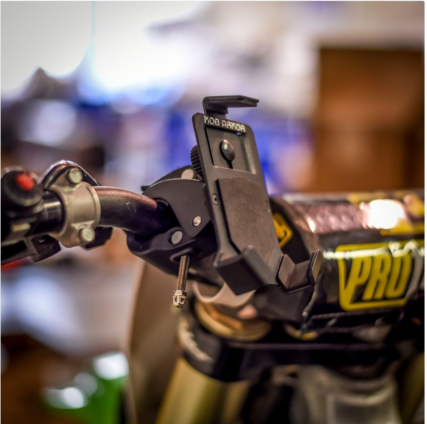
Figure 2: Components of the Mob Armor Switch Bar, showing the main holder and mounting clamp.
