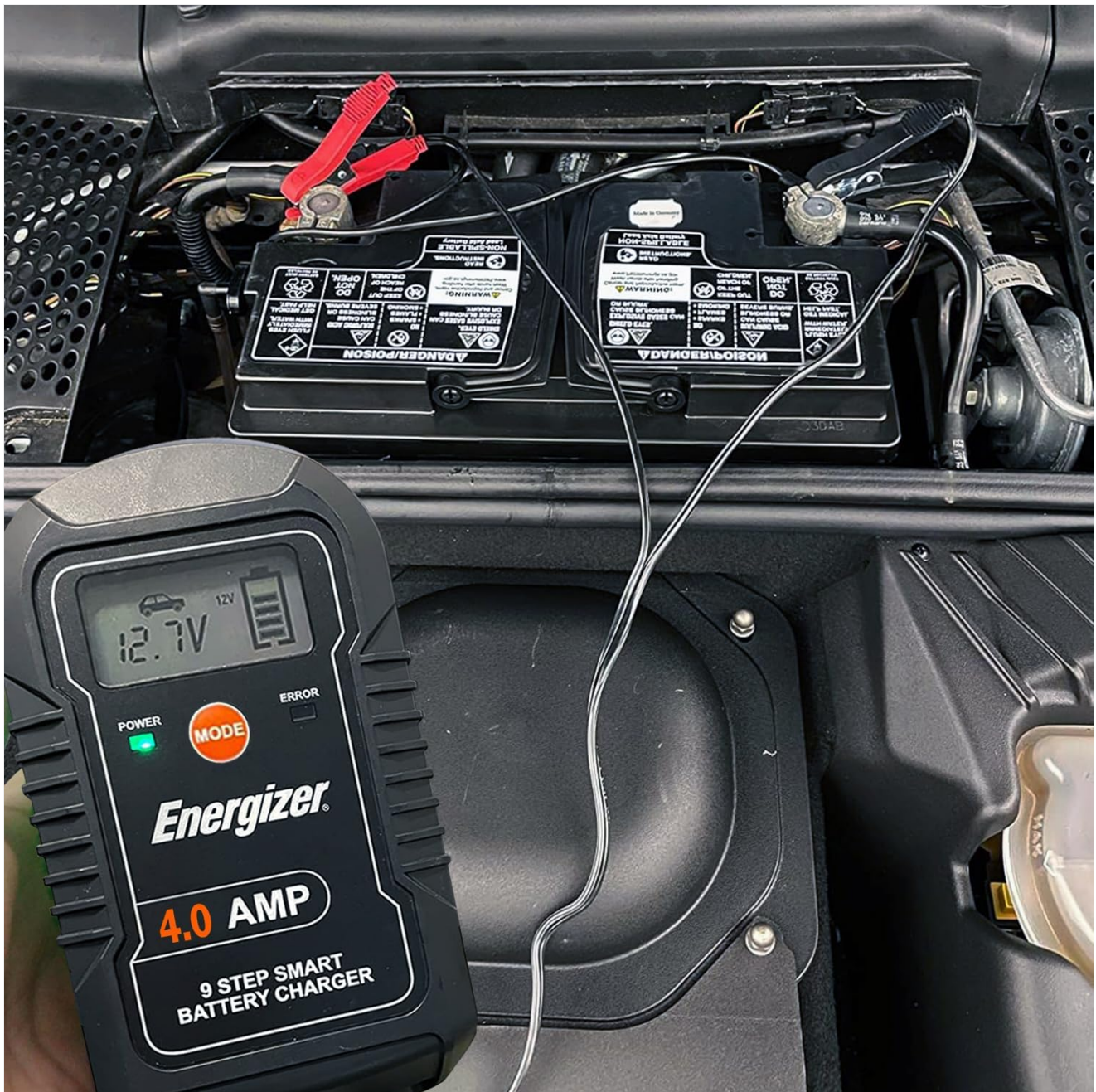
Image: The Energizer ENC4A charger connected to a car battery, showing the red clamp on the positive terminal and the black clamp on the negative terminal. The LCD displays the current battery voltage.
