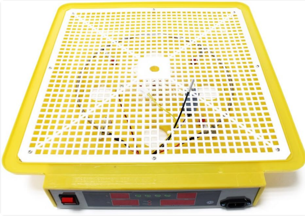
Figure 4.6: Top-down view of the incubator's internal structure, highlighting the protective grid over the fan and heating element, ensuring even heat distribution.
